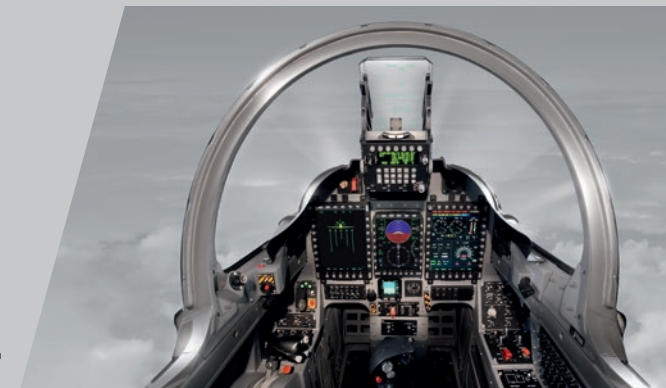
All-Glass cockpit & HOTAS: advanced HMI, similar to 4 th generation fighter airplanes.
